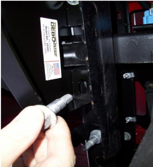
**Step 2.** Position your DEBO Step in line with the rear most bolt position. Re-install the rear most bolt all the way, but do not tighten at this time.
