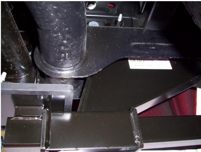
**Note:** Your DEBO Step will be at a slight angle downward when fully extended, due to the clearance between the step bar and the slide guide end plates. This design feature is what makes The DEBO Step® self locating!!
