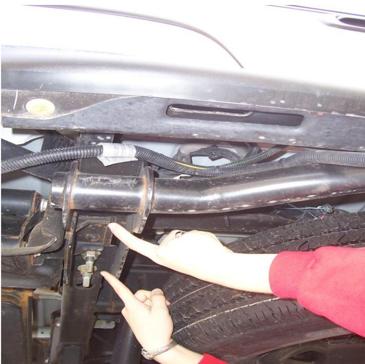
**Step 1.** The DEBO Step mounts on the driver side of the truck, using two of the existing M14 hitch frame mounting bolts.
