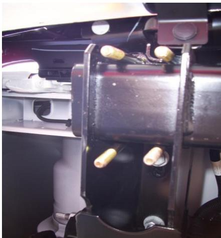
**Step 2.** Installing the other two bolts in the top plate will require tilting and maneuvering the top plate. Install the bolt toward the fender first, then install the bolt towards the spare tire.
