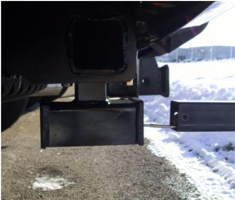
**Step 4.** Using the assembly instructions, insert the step bar through the slide guide and replace the rear bolt and nut.
