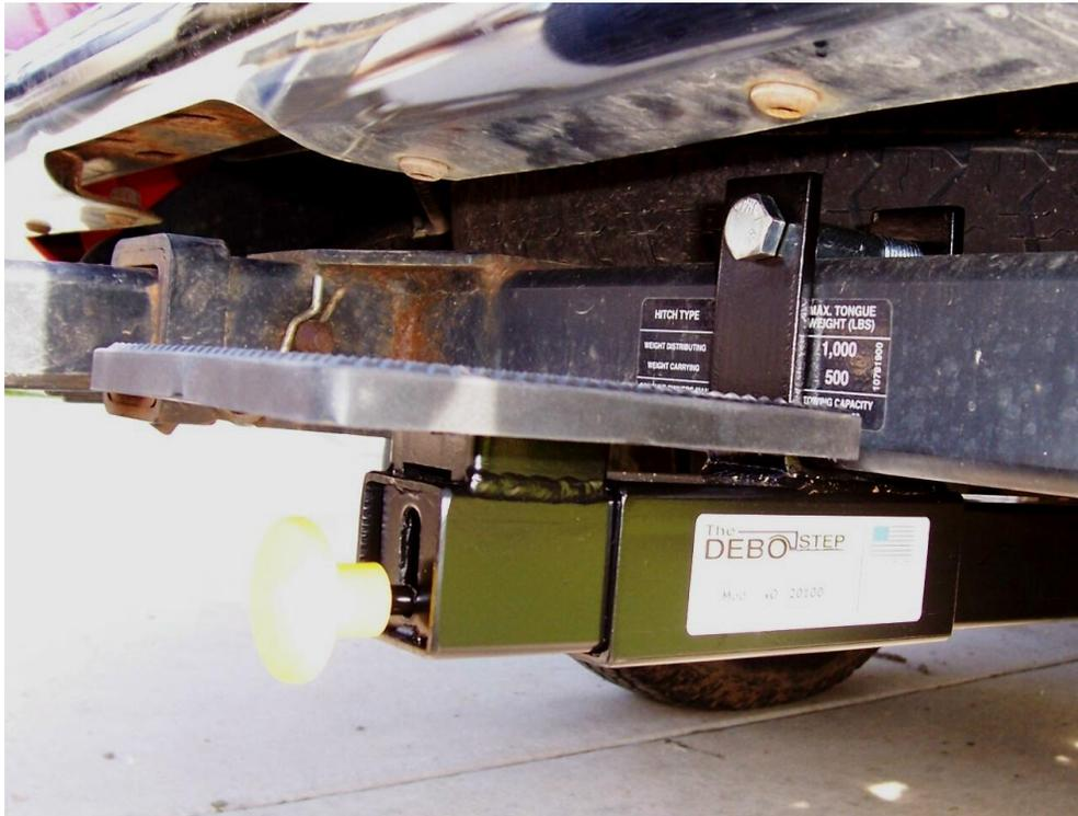
**Step 2.** Install the hex bolt in the cross holes of the u-bracket, as shown at left. The bolt can be installed in either direction.
