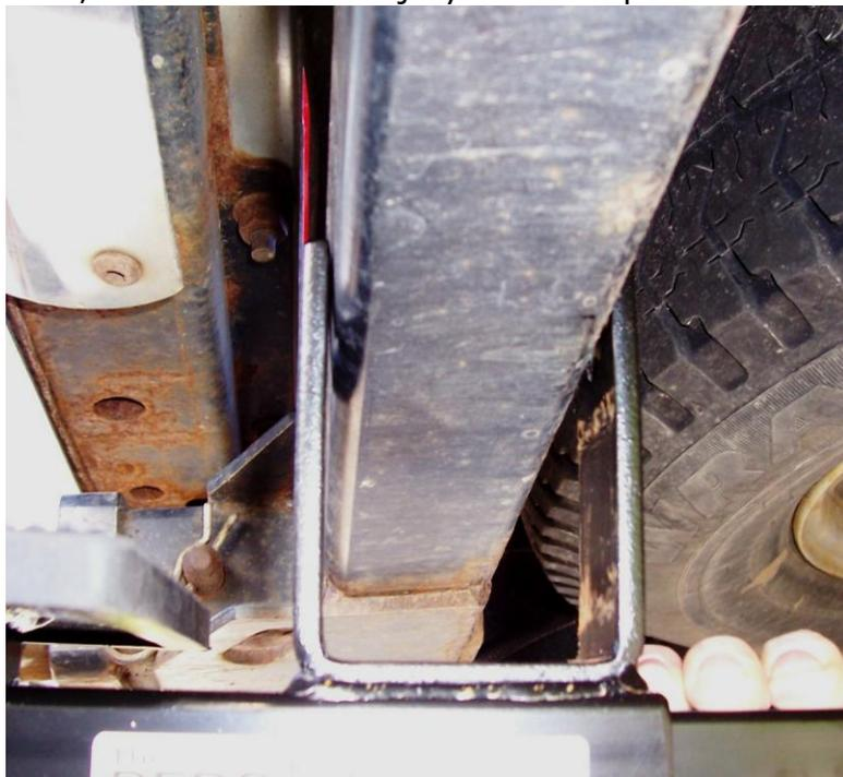
**Step 1.** The DEBO Step mounts on the hitch frame cross bar. The position on the crossbar depends on the truck and the hitch details.
