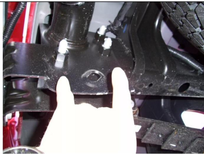
**Step 2.** The DEBO Step mounts on the driver side of the truck, on two of the cross frame bolts, and the slotted hole, as shown above.
