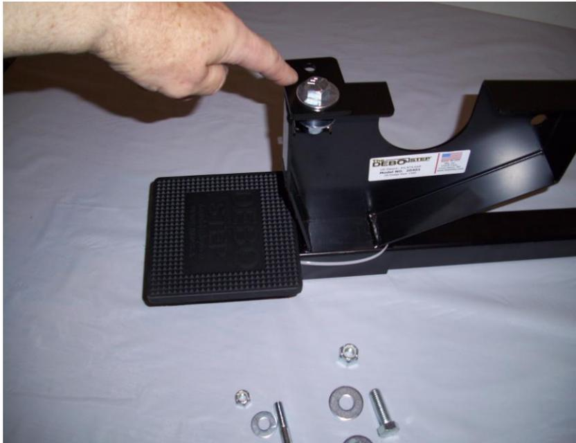
**Step 1.** Install the clamp plate as shown at left. Install a 1/2" washer on a bolt, insert from the bottom, up through the hole in the bracket and the clamp plate, install a washer and nylock nut. Tighten the bolt until snug, then back off one turn, so the clamp plate is loose and free to rotate.
