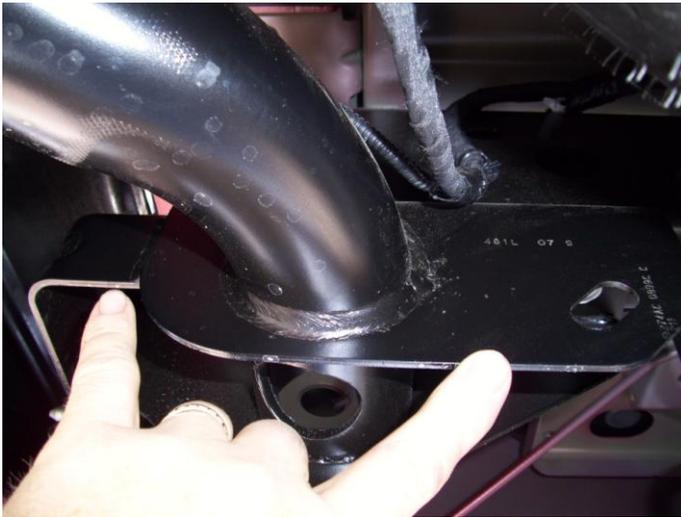
**Step 2.** Your DEBO Step mounts using the bumper bracket and the slotted hole in the hitch frame plate, as pointed to above, and shown installed below.
