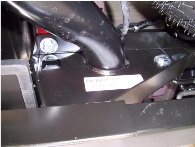
**Step 8.** Installation complete, slide the step in to the stowed position, check clearances to assure proper installation. Ready To Use!
