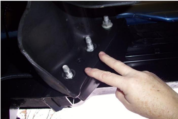
**Step 1.** The DEBO Step mounts on the drivers side of your truck, on the hitch frame as shown.
