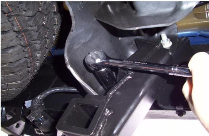
**Step 2.** Place the bracket over bolts, replace nuts and tighten securely!
