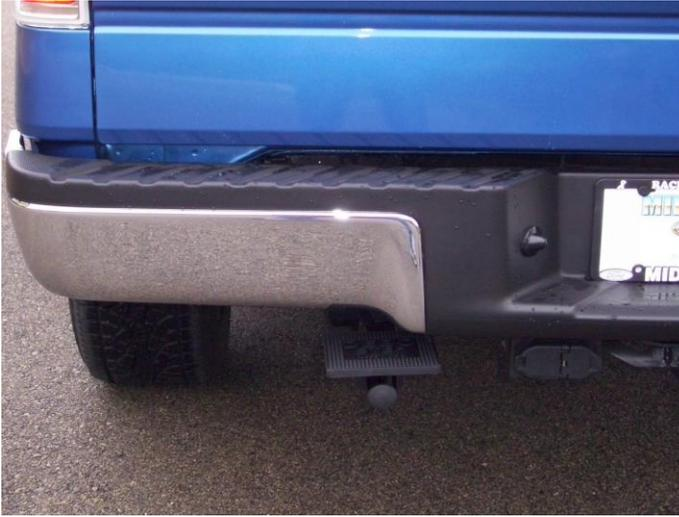
DEBO Step Installed, Stowed Position
