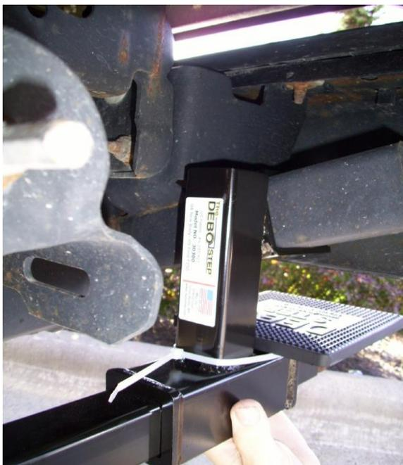
**Step 1.** The DEBO Step mounts on the drivers side of your truck, on the hitch frame cross bar.
