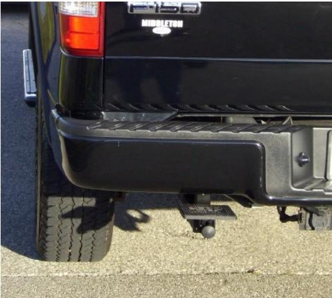
DEBO Step Installed, Stowed Position
