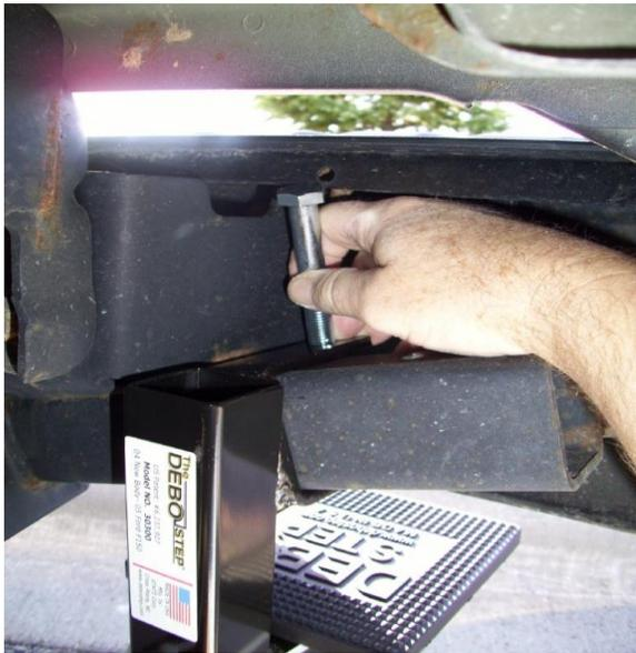
**Step 2.** Install the hex bolt in the cross holes of the u-bracket, as shown at left.
