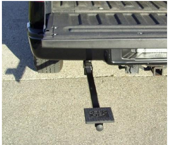
DEBO Step Extended for use with tailgate down.
