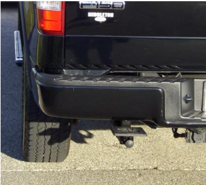
DEBO Step Installed, Stowed Position (04 New Body only, 04 Heritage use 30400)
