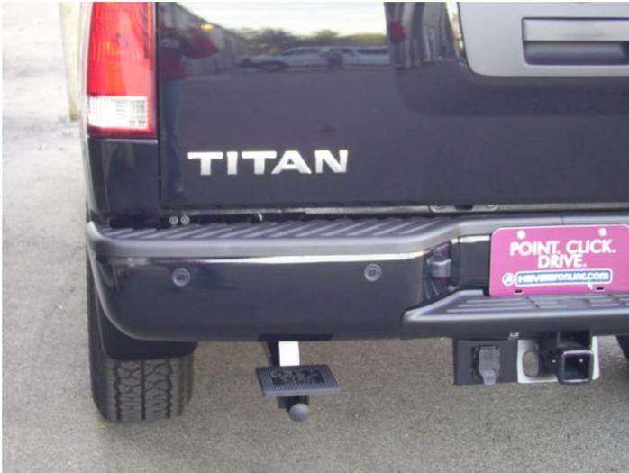
DEBO Step Installed, Stowed Position
