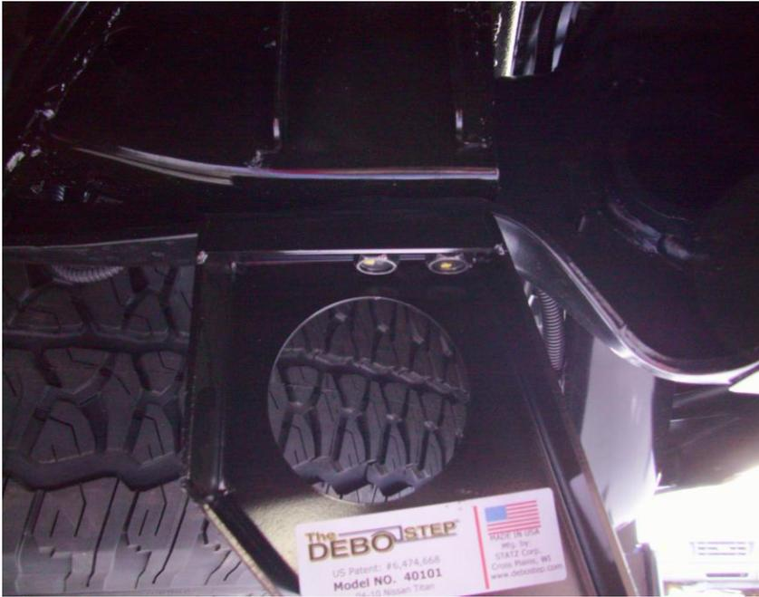
**Step 2.** Position The DEBO Step mounting bracket in place as shown at left.
