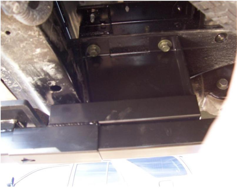
**Step 2.** Position The DEBO Step mounting bracket in place as shown at left and above, align holes, and re-install the (2) M12 bolts.
