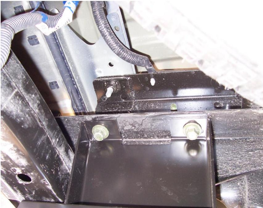
**Step 1.** The DEBO Step mounts on the driver side of the truck, using two of the existing M12 hitch frame mounting bolts as shown at left.
