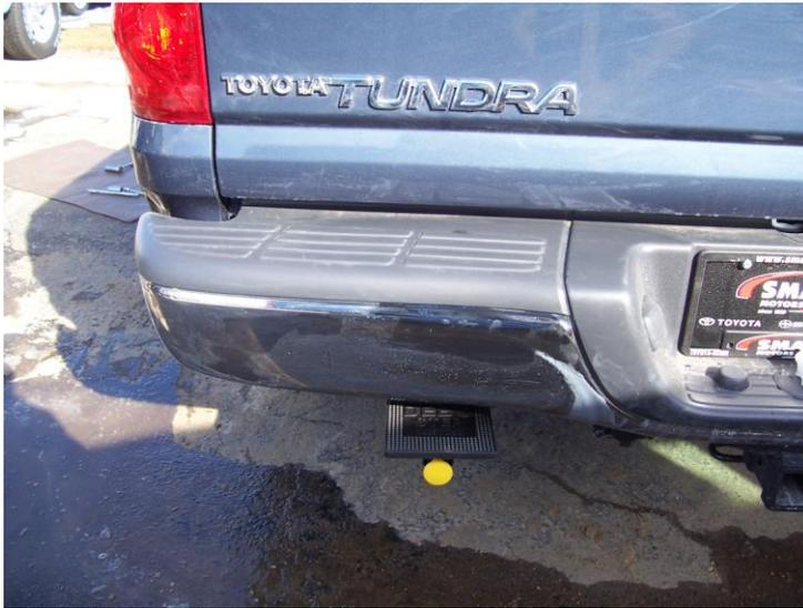
DEBO Step Installed, Stowed Position
