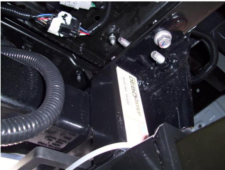
**Step 1.** The DEBO Step mounts on the drivers side of your truck, on the hitch frame cross bar.
